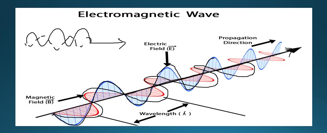
• The speed c of the electromagnetic wave in vacuum is related to  $\mu$  and  $\varepsilon$  (the free space permeability and permittivity constants) as follows:
