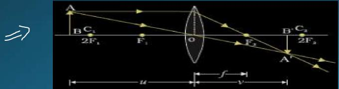
• When an object is at the center of curvature, the real image is formed at the other center of curvature.
