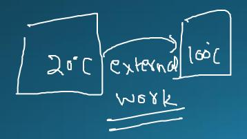
Kelvin's Statement It is impossible to obtain a continuous supply of work from a body by cooling it to a temperature below the coldest of its surroundings.
