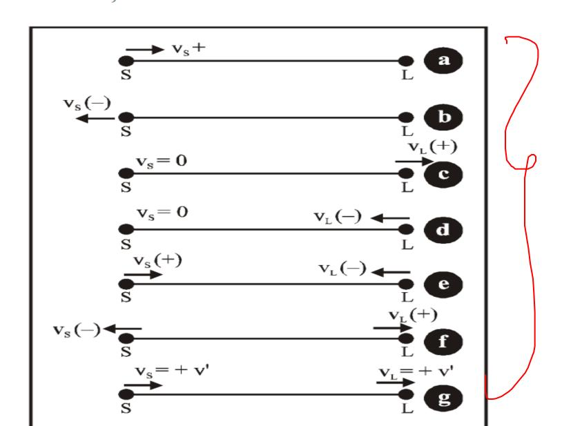
$$v' = \frac{\left(v - v_L\right)}{v} v \quad i.e. \ v' < v$$
