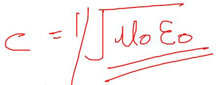
• The speed c of the electromagnetic wave in vacuum is related to  $\mu$  and  $\varepsilon$  (the free space permeability and permittivity constants) as follows:
