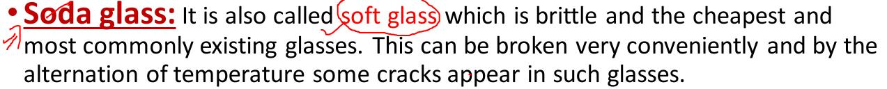
Low Melting Point [Na20. Coo. GSiO2] Bottle, Test Tube, Windows
