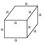
Diagonal of a cube =  $\sqrt{3} \times \text{one side} = \sqrt{3}a$
